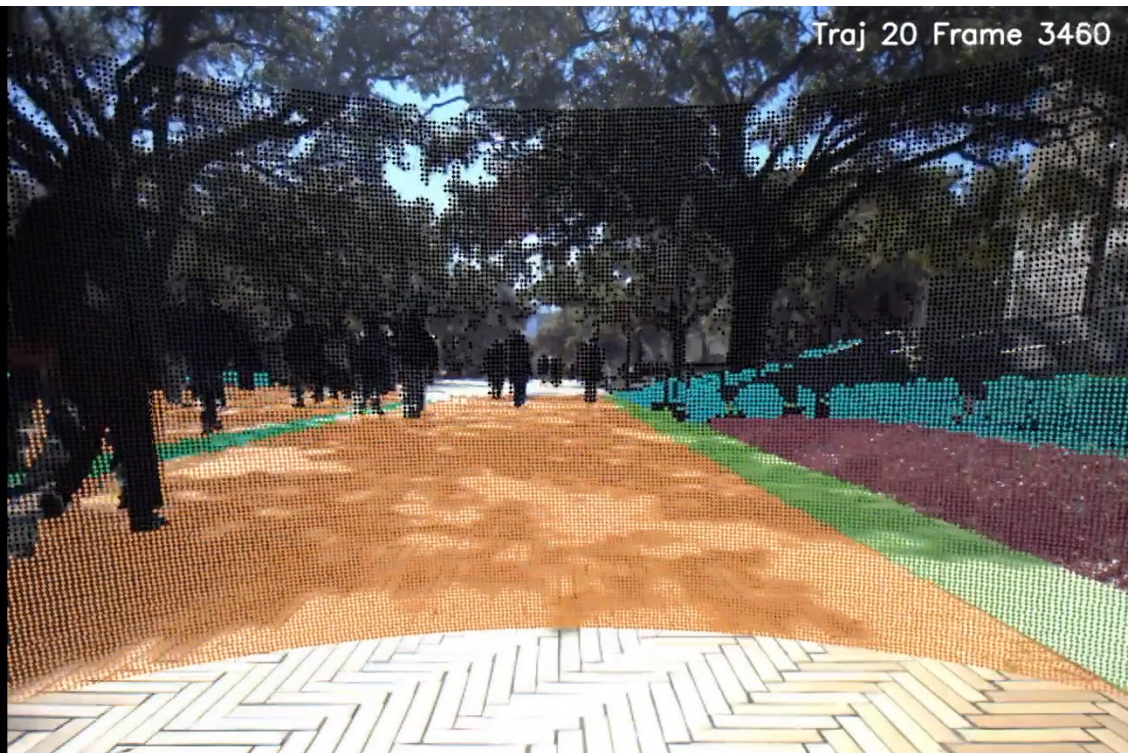
Terrain Annotations from 3D LiDAR Projected on RGB Image
